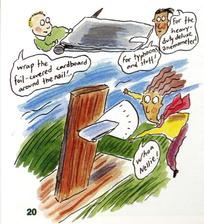
aluminum foil. Tape the ends together and tape it to the nail. This flap will be heavier than the first one and will be useful for measuring stronger winds. Calibrate your second anemometer just as you did the first, but for stronger winds.
